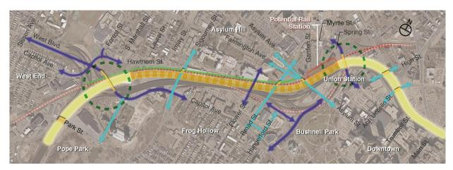
In this alternative, the railroad would again be relocated to the north of the highway to allow I-84 to be lowered below grade from
